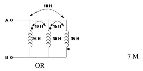
6. a) Determine the Y- parameters from the equivalent circuit for the given two-port network in Figure
